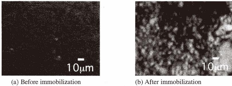
Fig. 1. Surface of the sensor chip (a) before and (b) after injection of *S. enteritidis* cells and washing with PBS and water. Into the flow cell equilibrated with PBS, 0.5 ml of the cell suspension was injected at a flow rate of 0.1 ml/min. After the injection, the flow was stopped for 20 min to immobilize bacterial cells on the surface of the sensor chip. The excess bacterial cells were removed by washing the flow cell with PBS at a flow rate of 0.1 ml/min.
