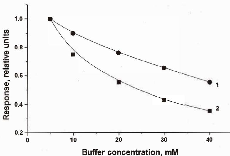
Fig. 3. Dependence of the output of the formaldehyde specific conductometric (1) and potentiometric (2) biosensors on the buffer concentration of the sample as measured in phosphate buffer, pH 7.7, at a formaldehyde concentration of 50 mM.
