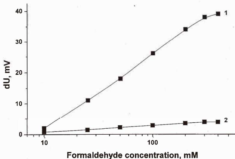
Fig. 4. Calibration curves (in semilogarithmic scale) for formaldehyde determination. Biosensor based on ISFETs. Steady-state responses were measured in 10 mM tris-HCl buffer, pH 7.7 (1) and 10 mM phosphate buffer, pH 7.7 (2). The same results were also obtained for biosensors based on conductometric transducers.
