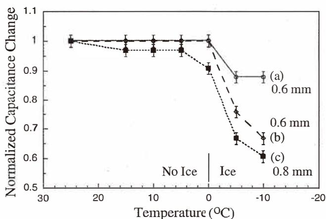
Fig. 12. Capacitance change of the diaphragm versus temperature for two different operational modes and ice film thicknesses: (a) continuous drive, 0.6-mm-thick ice layer; (b) intermittent drive, 0.6-mm-thick ice layer; and (c) intermittent drive, 0.8-mm-thick ice layer.
