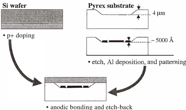
Fig. 5. Schematic illustration of sensor fabrication using a two-mask process.
