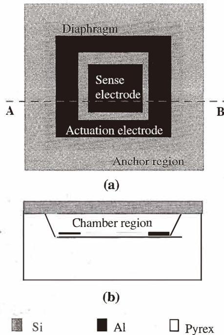
Fig. 1. Design concept of microfabricated ice detection sensor using a p+ silicon membrane: (a) plan thru-view; and (b) cross section across dashed line AB.
