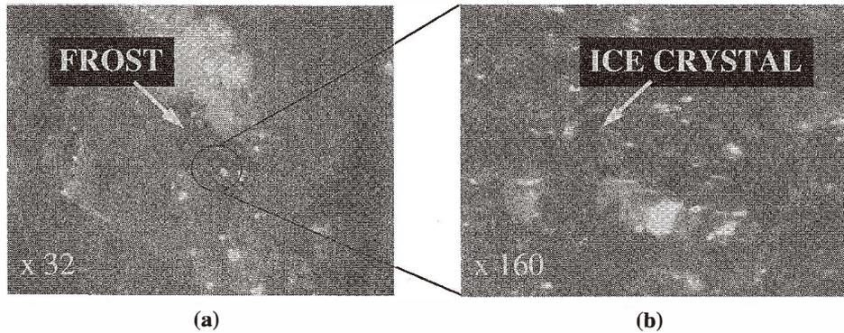
Fig. 11. Optical photographs (a): frost formation on an aluminum substrate at  $-8^{\circ}\text{C}$ ; and (b) close-up showing discrete ice crystals arranged in a columnar-like structure.
