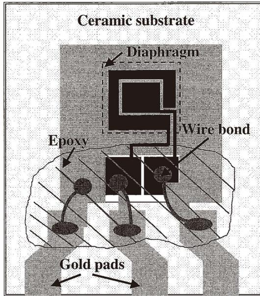
Fig. 6. Plan through-view of the final sensor package. The epoxy protects the bond wires and seals the chamber region watertight from the ambient.
