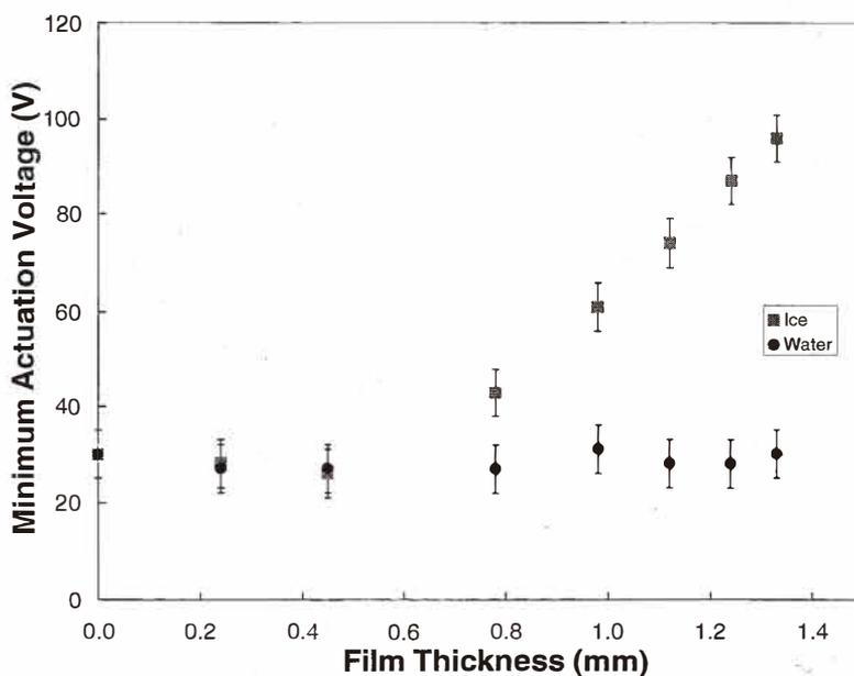
Fig. 9. Minimum diaphragm actuation voltage versus ice/water film thickness. The presence of water does not measurably affect the effective diaphragm stiffness.
