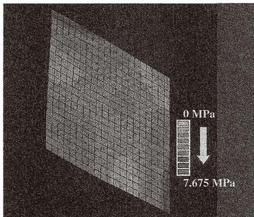
Fig. 3. FEA model of von Mises stress distribution on sensor diaphragm. The maximum stress regions are located at the centers of the diaphragm edges.
