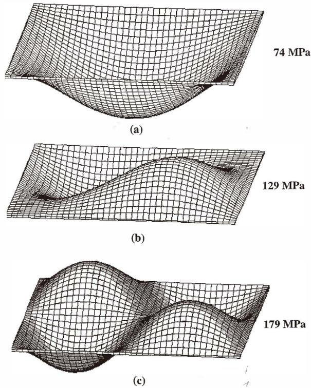
Fig. 4. FEA results showing the first three buckled mode shapes and the corresponding stress load required: (a) first mode; (b) second mode; and (c) third mode.
