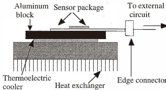
Fig. 7. Experimental setup for testing the operation of ice detection sensor. The external circuit connects to the capacitance measurement circuit.
