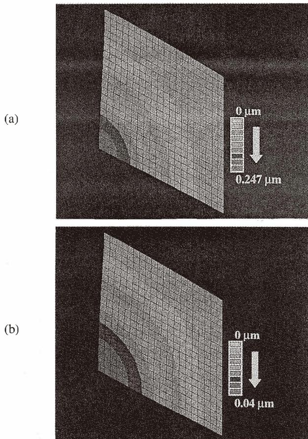
Fig. 2. FEA results showing diaphragm deflection under various conditions: (a) ice/water-free diaphragm with 50 V electrostatic actuation; (b) 10-mm-thick water layer only.
