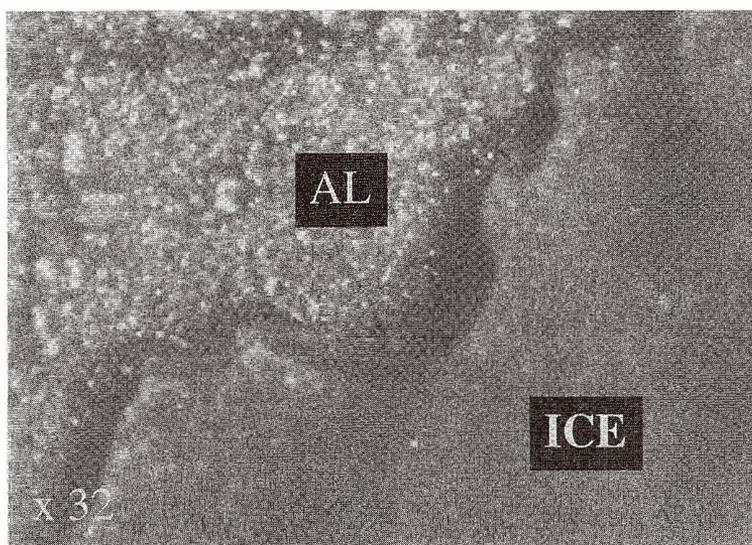
Fig. 10. Plan view micrograph showing clear ice formation at  $-5^{\circ}\text{C}$ .
