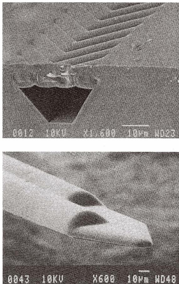
Fig. 6. SEM views of a sealed microchannel in bulk silicon and of the back of a drug delivery probe containing two such channels.
