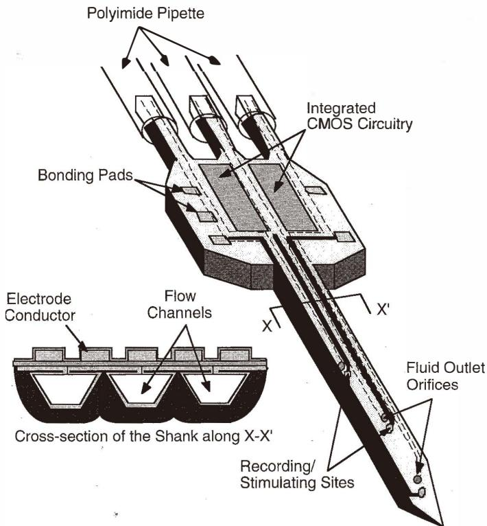
Fig. 5. Diagram of a probe containing microchannels for drug delivery as well as electrical stimulating and recording sites.
