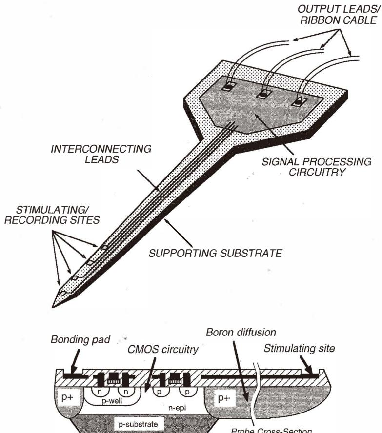
Fig. 1. Overall structure of a multisite probe for interfacing with tissue at the cellular level.
