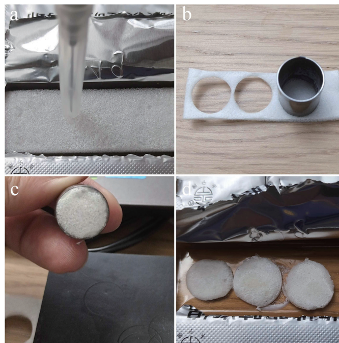
Fig. 1. (Color online) (a) Moisturization of the gelatin sponge (GS) strip using the end cap of a syringe to smooth the saline drops on the surface of GS strip. (b) A 15-mm-diameter circular knife was used to cut the GS strip into circular pieces. (c) Polymerization of GS-NbCG. (d) GS-NbCG specimens.
