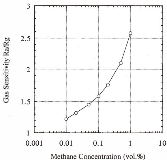
Fig. 11. Relationship between gas sensitivity and methane concentration. The heater was operated under the same conditions as in Fig. 9.
