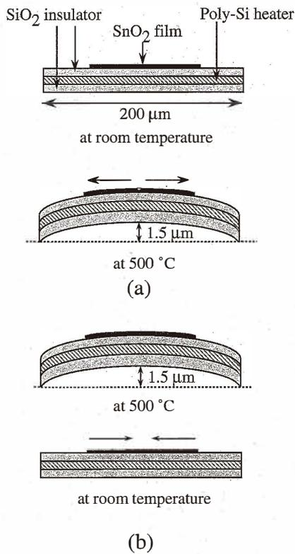
Fig. 13. Schematic cross-sectional views of two sensors at  $500^\circ\text{C}$  and at room temperature. (a) is the C-sensor and (b) is the N-sensor.
