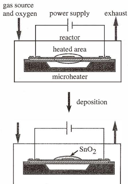
Fig. 6. Selective deposition by the novel MOCVD method.
