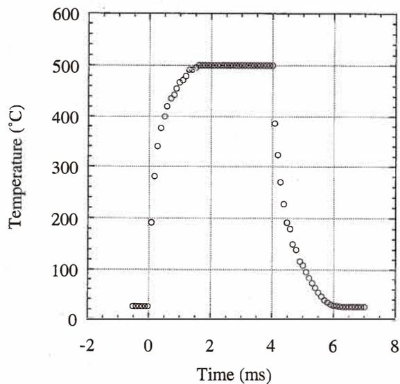
Fig. 7. Thermal response of the N-sensor when heated to 500°C and cooled to room temperature.
