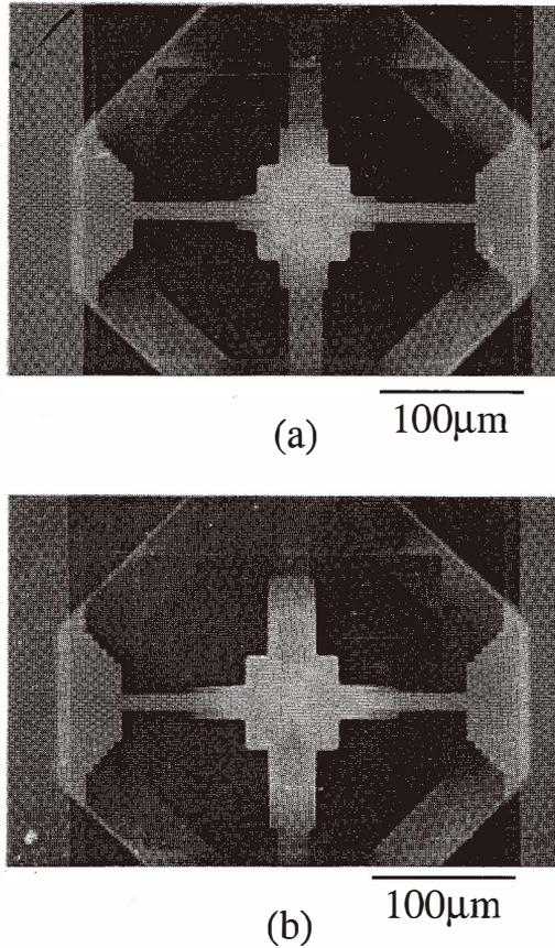
Fig. 8. SEM images of two sensors after deposition of SnO<sub>2</sub> using the novel method. The temperatures of the heater are (a) 500°C and (b) 600°C.
