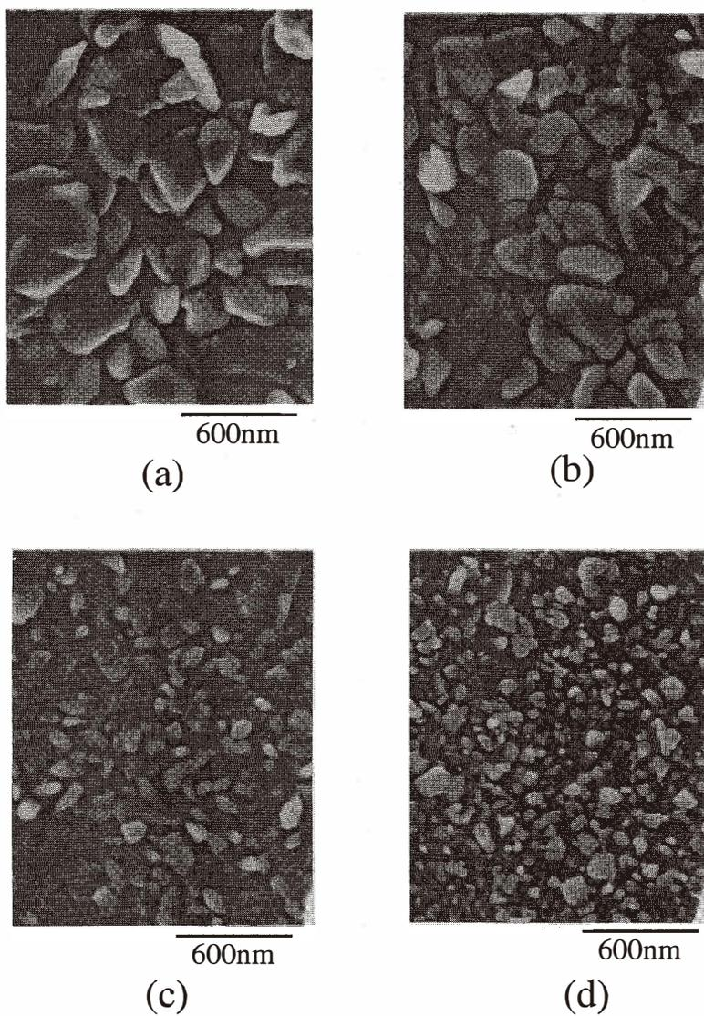
Fig. 14. SEM images of SnO<sub>2</sub> films with different deposition times of (a) 180 s, (b) 140 s, (c) 100 s and (d) 60 s.
