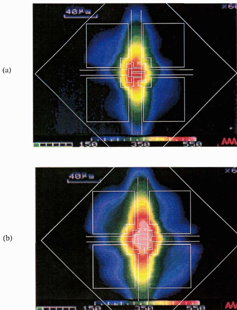
Fig. 5. Temperature distribution on the microheater. The temperatures at the center of the heater are (a) 500°C and (b) 600°C.
