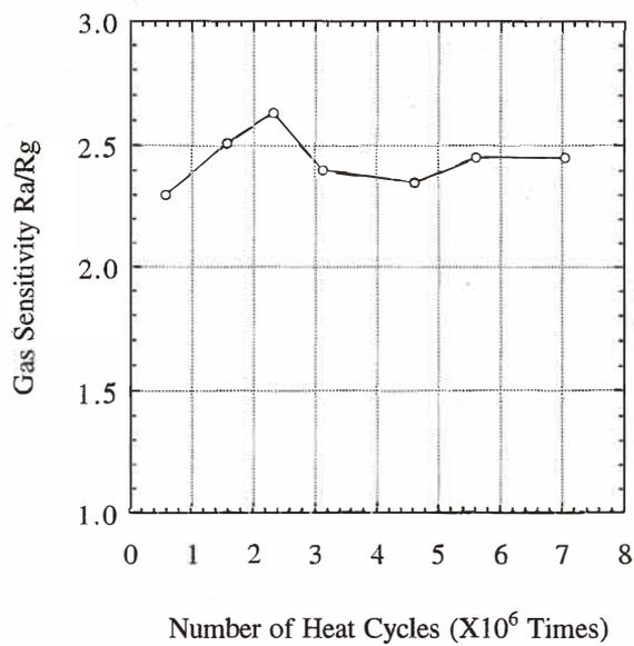
Fig. 10. Time dependence of the gas sensitivity of the N-sensor to 1% methane.
