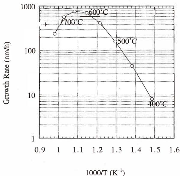
Fig. 4. Dependence of the growth rate of SnO<sub>2</sub> film on substrate temperature. Films were deposited using the hot-wall MOCVD method.
