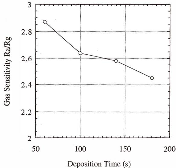
Fig. 15. Dependence of gas sensitivity to 1% methane on deposition time. The heater was operated under the same conditions as in Fig. 9.
