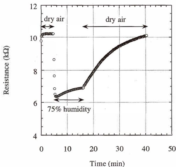
Fig. 12. Response of the N-sensor to 75% humidity.
