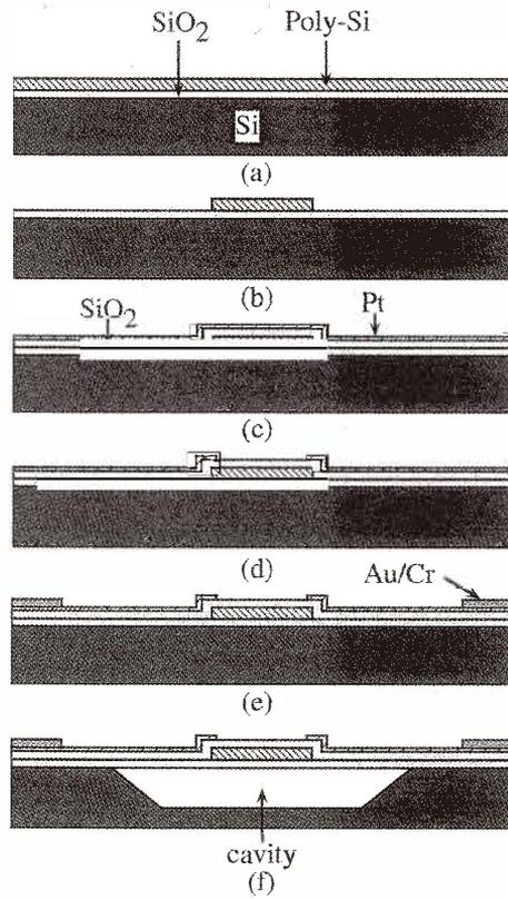
Fig. 1. Fabrication of the microheater.
