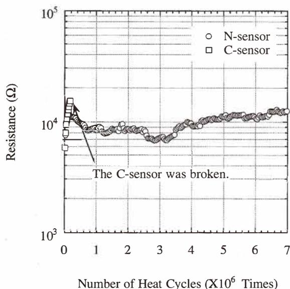
Fig. 9. Time dependence of the resistance of two sensors. The heaters were intermittently operated. One heat cycle consisted of 500°C for 100 ms followed by room temperature for 100 ms.
