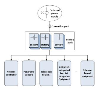
Fig. 5. (Color online) Designed power supply scheme of panoramic acquisition platform system.
