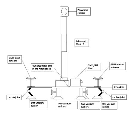
Fig. 7. Structural design of the panoramic platform.
