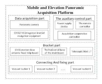
Fig. 1. Overview of the mobile elevating panoramic acquisition platform.
