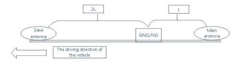
Fig. 2. Illustration of the GNSS double-antenna positions.
