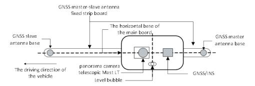
Fig. 3. Plane positional diagram of each part of the bracket.
