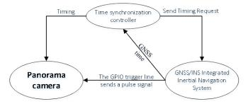
Fig. 6. Data acquisition by pulse triggering GNSS time and controlling synchronization.
