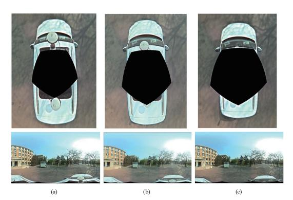
Fig. 10. (Color online) Panoramic renderings obtained with different heights of the panoramic camera during shooting. Top: panoramic camera; bottom: corresponding panoramic photograph for panoramic camera heights of (a) 2.5, (b) 2.7, and (c) 2.9 m.
