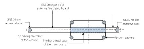
Fig. 4. (Color online) Positional diagram of the six vacuum suction cups.
