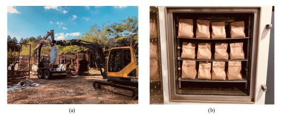
Fig. 3. (Color online) (a) Comminution of each forest residue pile and (b) oven drying of sample wood chip.
