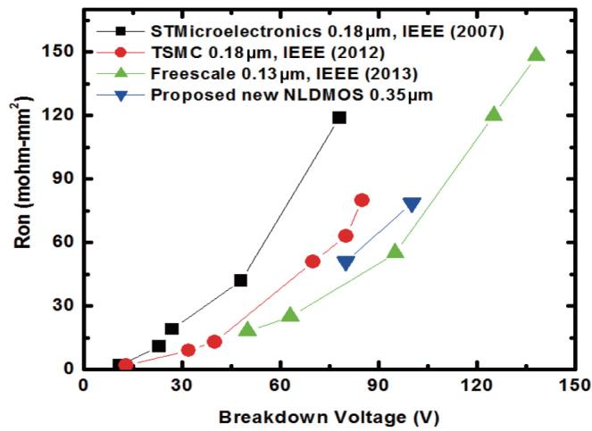
Fig. 6. (Color online) Comparison of benchmark off-state breakdown vs on-state resistance ( $R_{on}$ ) for different technologies.
