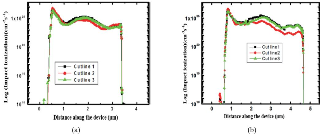
Fig. 3. (Color online) Surface impact ionization distributions of proposed (a) 80 and (b) 100 V NLDMDOS unit cells.
