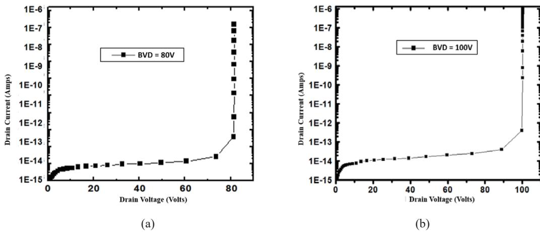
Fig. 4. Breakdown curves for proposed (a) 80 and (b) 100 V NLDMDOS unit cells.
