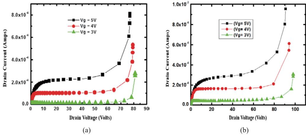
Fig. 5. (Color online) SOA curve for proposed (a) 80 and (b) 100 V NLDMOS unit cells.
